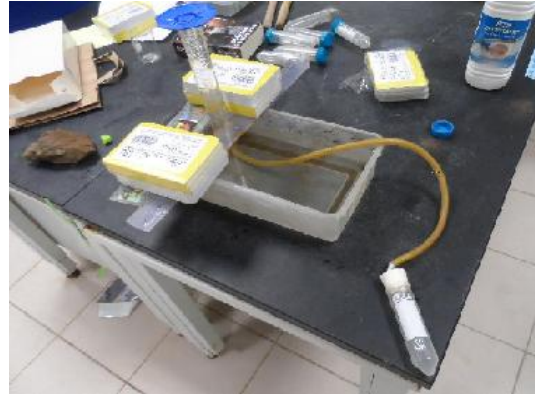
FIG. 2. APPARATUS USED TO MEASURE A VOLUME OF GAS FROM SOIL AND ACID REACTION
